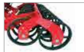
Actipress Twin ø 560 mm 220 kg/m (up to 250kg/m with soil)
