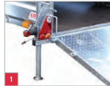
Prop stands to support the trailer when loading vehicles.
