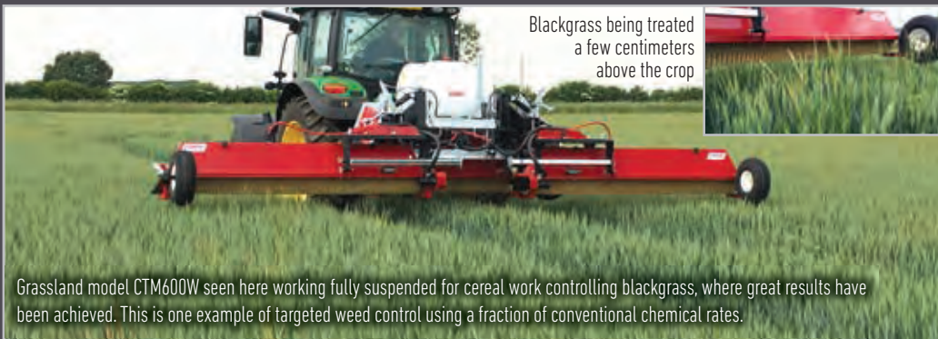
Hydraulic 'float' setting allows the unit to follow field contours.
