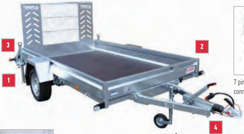
Monoque construction with 'A' frame drawbar, Al-Ko suspension, one piece axle (1300kg) featuring rubber progressive action with excellent dampening. All protected with hot dipped galvanising for long life.
