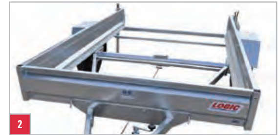
Monoque construction with 'A' frame drawbar, Al-Ko suspension, one piece axle (1300kg) featuring rubber progressive action with excellent dampening. All protected with hot dipped galvanising for long life.
