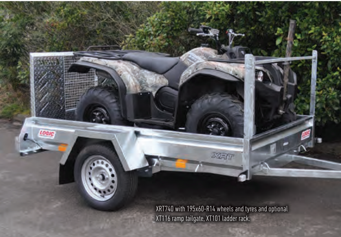
1 Optional XT116 metal loading ramp/tailgate, for loading ATVs, garden machinery, etc.
