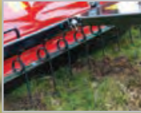
MSP120WT fitted with tine bar, seen here (right) breaking up 'rained in' horse droppings.
