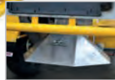
Optional PDS210 disc shroud to further reduce spread width.
