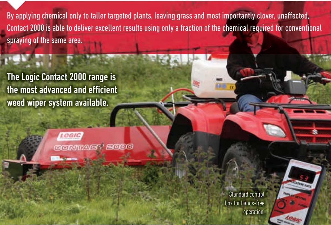
Height adjustment is spring-assisted to allow the machine to be quickly and easily set to the correct working height for the weed infestation being treated.
