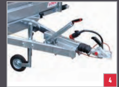
Overrun brakes with safety breakaway cable, handbrake and jockey wheel.
