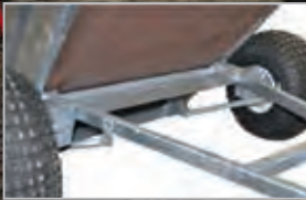
Spring assisted tipping mechanism.
