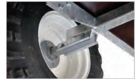
Bolt-in stub axle to allow easy maintenance or replacement when the time comes, without disturbing the galvanising protection.
