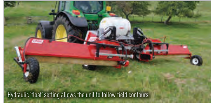
The two outer wings have a resettable, hydraulic break-back facility to protect the machine against damage from unforeseen obstacles.
