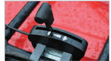
Throttle control is positioned close to hand and allows instant build up from idle, when required. Brush engagement is controlled via a centrifugal clutch which starts the brush when the engine revs are increased.
