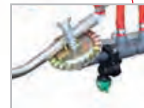
Break-back clutch to protect spraylines in operation or fold up in transport mode.
