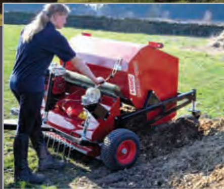
The manual unloading winch is easy to operate and features a geared system with controlled release.
